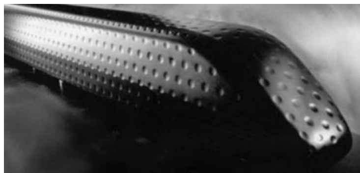
Fig. 2. The high-speed train model with dimpled surface relief
