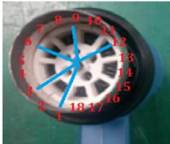
Figure 2. Velocity distribution along the radial lines that correspond the axial positions: 1 (no hole); 3, 12 (big holes), 6, 9 (small holes) (velocity should be multiplied by scaling factor 10)
